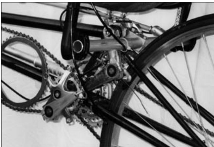
Figure 2. Close-up of the arm powered rowing/steering mechanism
